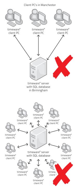
In this example we have client PC's that are located in Manchester and a timeware® server in Birmingham. This setup would cause a massive amount of problems with connectivity that would result in an unusable system. It is NOT recommended to have the client PC's connecting over long distances. Instead, it is recommended to have the client and server be on the same local network.
